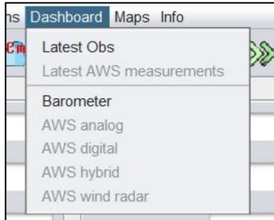
**Latest Obs** - Display details from the latest observation. Observation less than 12 hours old displayed with a Green background color. More than 12 hours but less than 24 with yellow background. Observations older than 24 hours with a red background.
