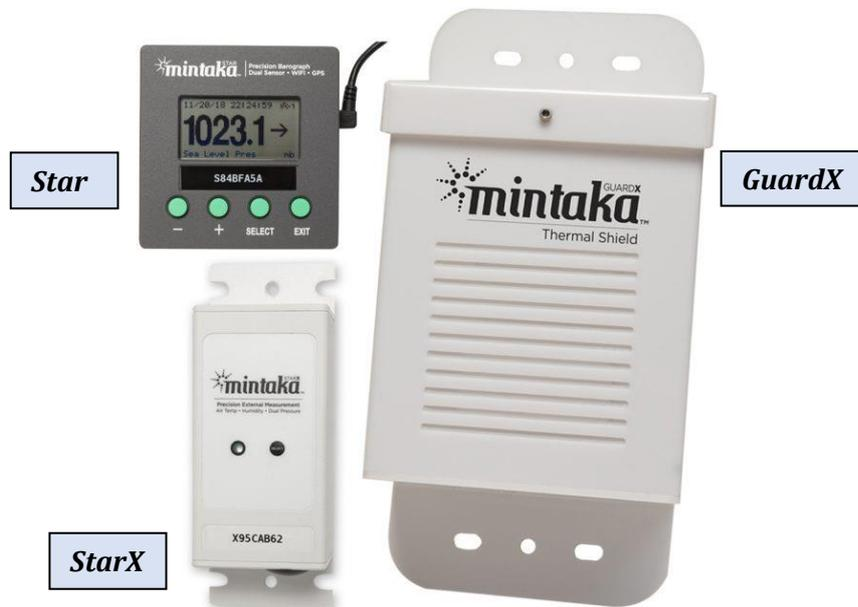
**Mintaka StarX** is designed as an outside unit installed on a ship's bridge wing. It measures station pressure, air temperature and relative humidity, then communicates the data to the Mintaka Star on the bridge via WiFi every 5 minutes. Data from the StarX and GPS data from the Star are pushed via USB cable to the ship's computer and into TurboWin+. It is fully independent of ships power. Runs on a lithium battery lasting 6 to 9 months.
